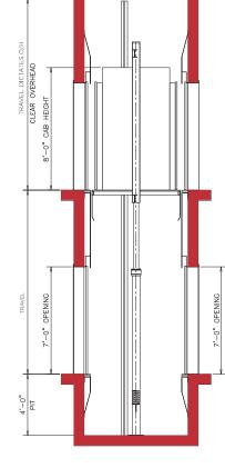
**Description:** The design utilizes two hydraulic single stage jacks, located on each side of the platform and installed directly on the pit floor. Opening configuration available in walk-thru and/or staggered. Staggered doors are required to accommodate the ambulance size stretcher.
